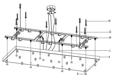
In Instruction This fixture is provided with Safety Cables. The Safety Cable provides a back up system the mounting frame and the installation hardware. It is essential that the Safely Cable be properly installed. The Cable must be secured to a STRUCTURAL MEMBER of the building, and not to the outlet box. The Cable must be terminated with Steel cable lock kit specifically sized for the Cable per the following steps:
