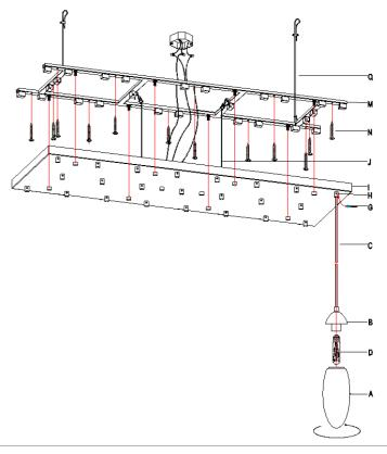
In Instruction: This fixture is provided with Safety Cables. The Safety Cable provides a back up system the mounting frame and the installation hardware. It is essential that the Safely Cable be properly installed. The Cable must be secured to a STRUCTURAL MEMBER of the building, and not to the outlet box. The Cable must be terminated with Steel cable lock kit specifically sized for the Cable per the following steps:
